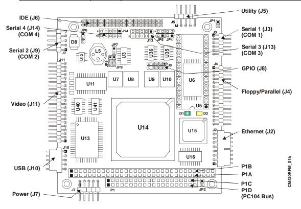
Figure 2-4. Connector Locations (Top View)
